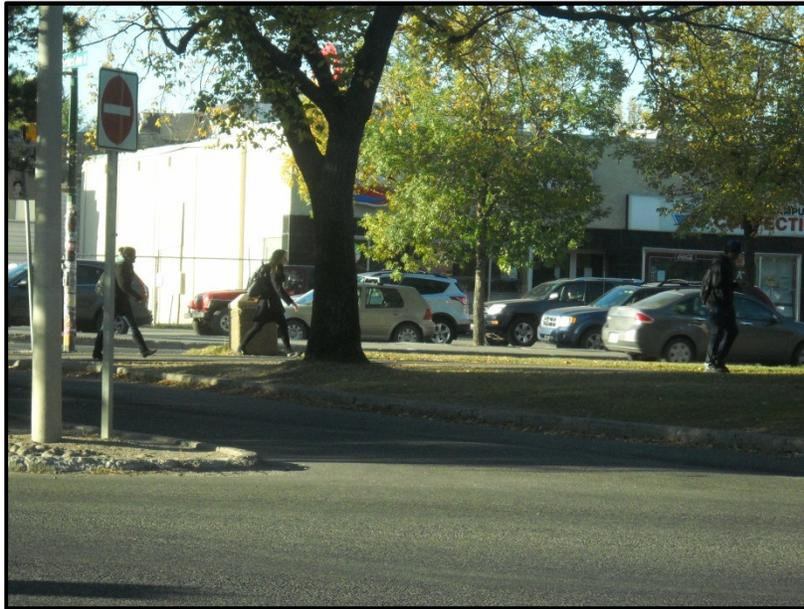
This sign makes it illegal for all vehicles to enter, but the intent is to prevent personal vehicles from driving along it while still allowing buses to access it. A tab should accompany the sign indicating “Except Buses” or similar. Alternatively, a sign similar to the one used at Bottomley Road indicating buses are permitted may be used.
